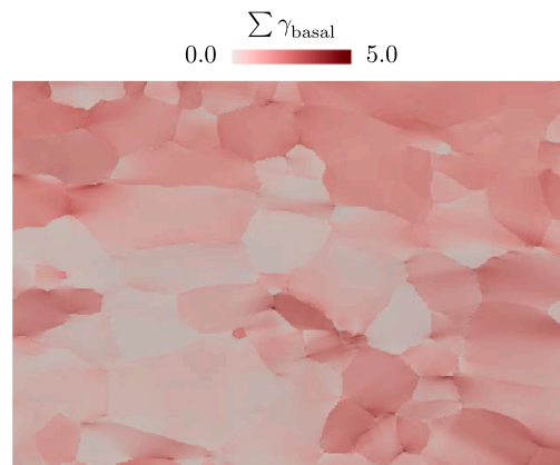
(b) Results of the Crystal Plasticity (CP) simulations: Magnitude of shear on all basal slip systems.
