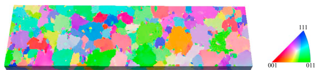
Fig. 34. 3D model obtained from serial sectioning Electron Backscatter Diffraction (EBSD) used for the Dual Phase (DP) steel simulations. The dimensions are 70.0 \mu\text{m} \times 20.0 \mu\text{m} \times 2.9 \mu\text{m} . Color indicates Inverse Pole Figure (IPF) along the horizontal loading direction.
